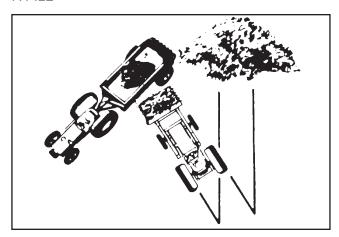
For faster loading, minimize the angle of turn and length of run between pile and spreader.
